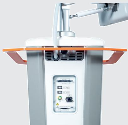
Connect to an external overhead screen using the easily accessible DVI port located on the media panel. The **MiraQ™ Cardiac** software has native support for configuring screen size and resolution.
